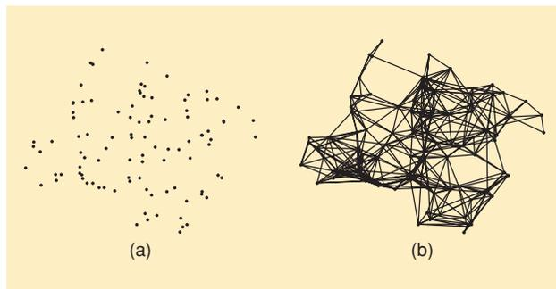
**[FIG1] Sensor localization: (a) the physical location of a collection of sensors may be represented as (b) a graphical model in which nodes correspond to the sensor node location variables and edges correspond to observed information, such as intersensor distance measurements from a subset of node pairs.**
