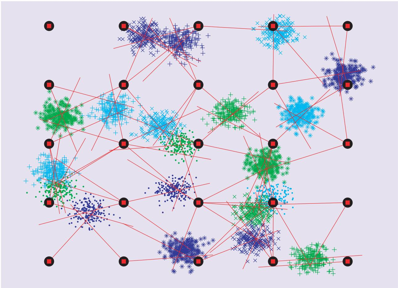
**[FIG2]** A snapshot of a typical data association scenario in a sensor network. Twenty five sensors (circle nodes) and the bearing-only measurements (line segments) are shown. Each cluster of samples represents the prior position distribution of one target.
