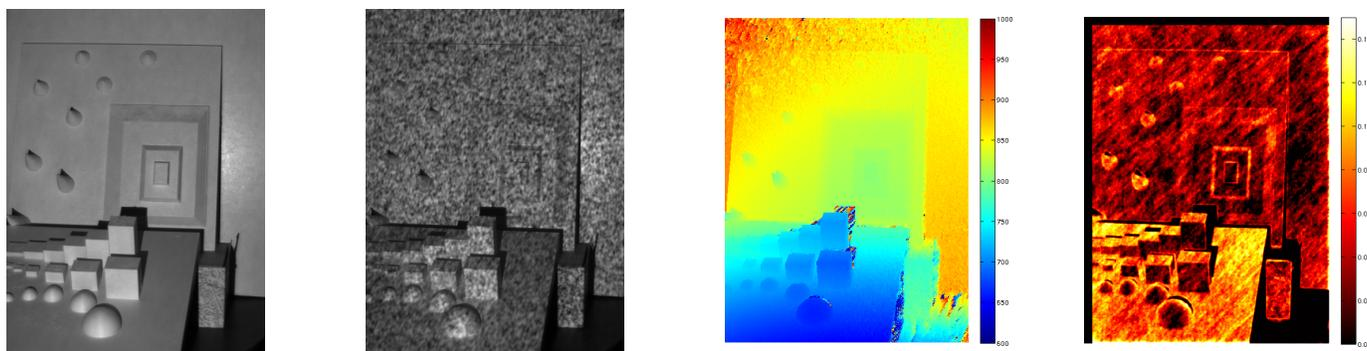
Fig. 13. Left-to-right, top row: an image of the scene, one of the projected patterns as capture, the range image, the pixelwise mutual information with respect to the pose, which initial uncertainty in the camera's  $xy$  plane. The main informative areas are the cones, and regions that face the  $x, y$  directions.
