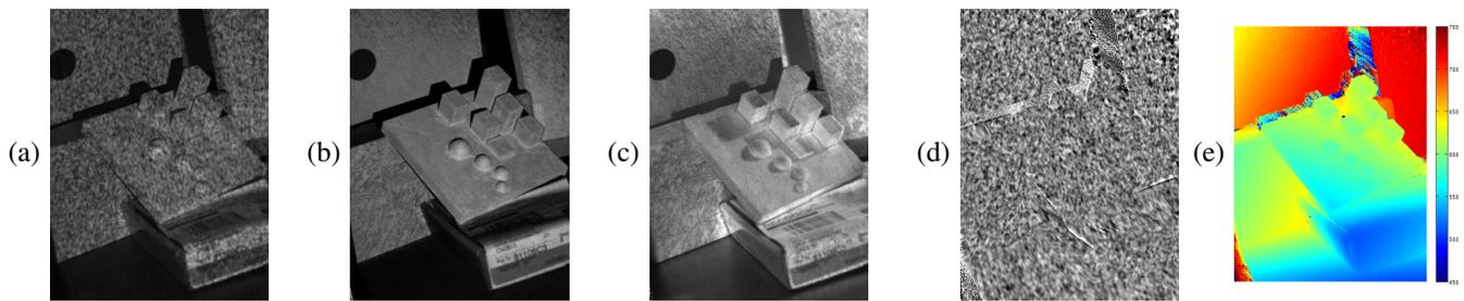
Fig. 3. Left-to-right: a)  $I_c$ , b) coefficients  $a$  and c)  $b$  from Equation 3 for the MAP-estimated range d)  $I_p$  in the camera image plane, e) the range image in millimeters. Note how parameter  $b$  captures scene illumination, whereas parameter  $a$  captures the reflectance coefficient of the surface with respect to the projector.
