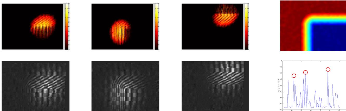
Fig. 12. Left-to-right, top row: the top 3 selected masks from a set of 60 masks, and the range image. Bottom row: a MAP estimated images for the 3 masks, used when estimating the MI for each pattern, followed by the average MI scores for the patterns. Red circles mark the patterns shown.
