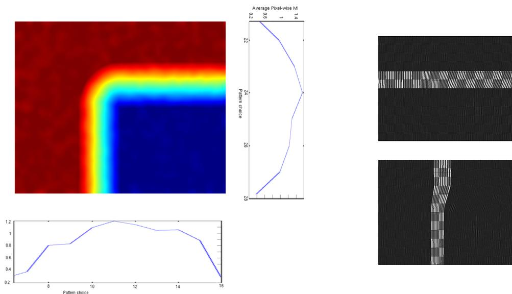
Fig. 11. Left: the depth image and the MI scores of vertical and horizontal stripe masks of the patterns with respect to pose estimation in the  $xy$  plane. Right: the top-scoring horizontal and vertical patterns, as seen when projected onto the scene. As can be seen, the patterns that were selected are the ones illuminating the edges and corner.
