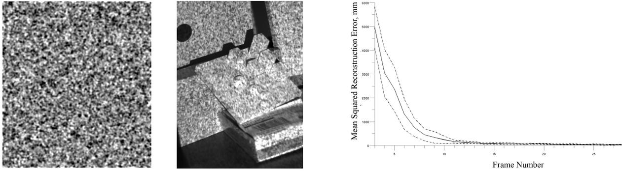
Fig. 5. Left-to-right: a projected Gaussian-smoothed pattern, a captured image, average reconstruction error as a function of the number of patterns used. Dashed lines mark the standard deviation over pattern sequences.
