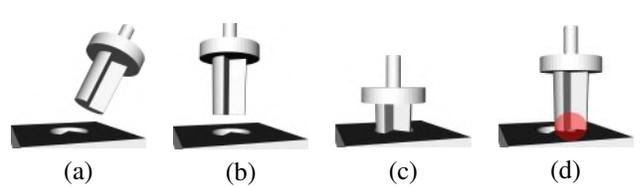
Fig. 3: An open-loop plan for part insertion. **a)** Initial (believed) position  $\mathbf{x}_S$ . **b)** Initial alignment. **c)** After insertion. **d)** Performing the open-loop plan for  $\mathbf{x}_S$  whereas the real initial pose is  $\mathbf{x}_T$  could result in a collision (shown in red), or task failure.
