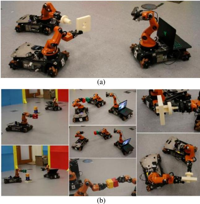
Fig. 1: (a) A team of robots assembling a peg into a hole. The rightmost robot carries a sensor to localize the assembly parts and provides feedback. The grasps, robot base/arm configurations, and the sensor position are all planned to avoid collisions *and* to position the sensor optimally for the task. (b) Example tasks - block stacking, block assembly, peg in hole.
